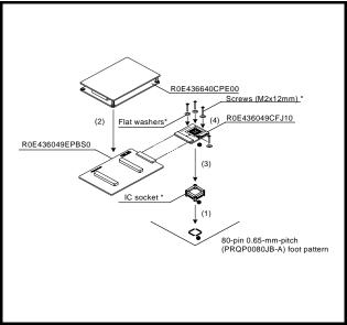
Figure 3 Connection procedure of the R0E436049CFJ10
